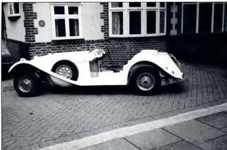
Above: Fitting the body was easier than expected and various shims were used to avoid the body rattling against the chassis. Below: Separate scuttle top also acts as a dash backing plate into which Roy fitted some Triumph Dolomite instruments.
