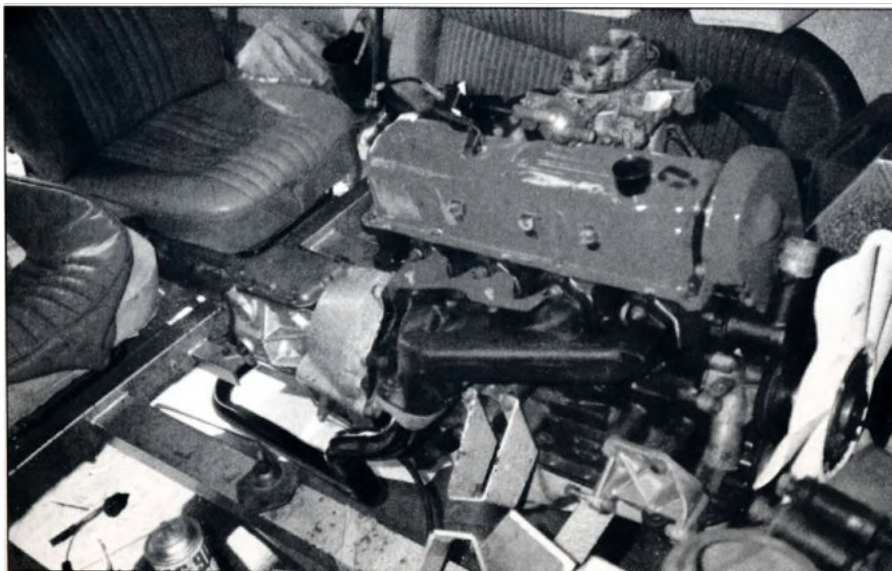
Above: This is the bodyshell as it arrived from Merlin. Quality of the mouldings was good and everything was carefully stored to prevent any flexing whilst the GRP was finally curing. Below: The 2-litre engine was stripped down and thoroughly inspected.
