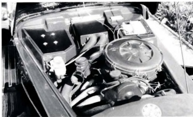
The underbonnet area is tailored specifically for the OHC engine. Note the way the pedal box is hidden and the battery stored above the passenger footwell.
