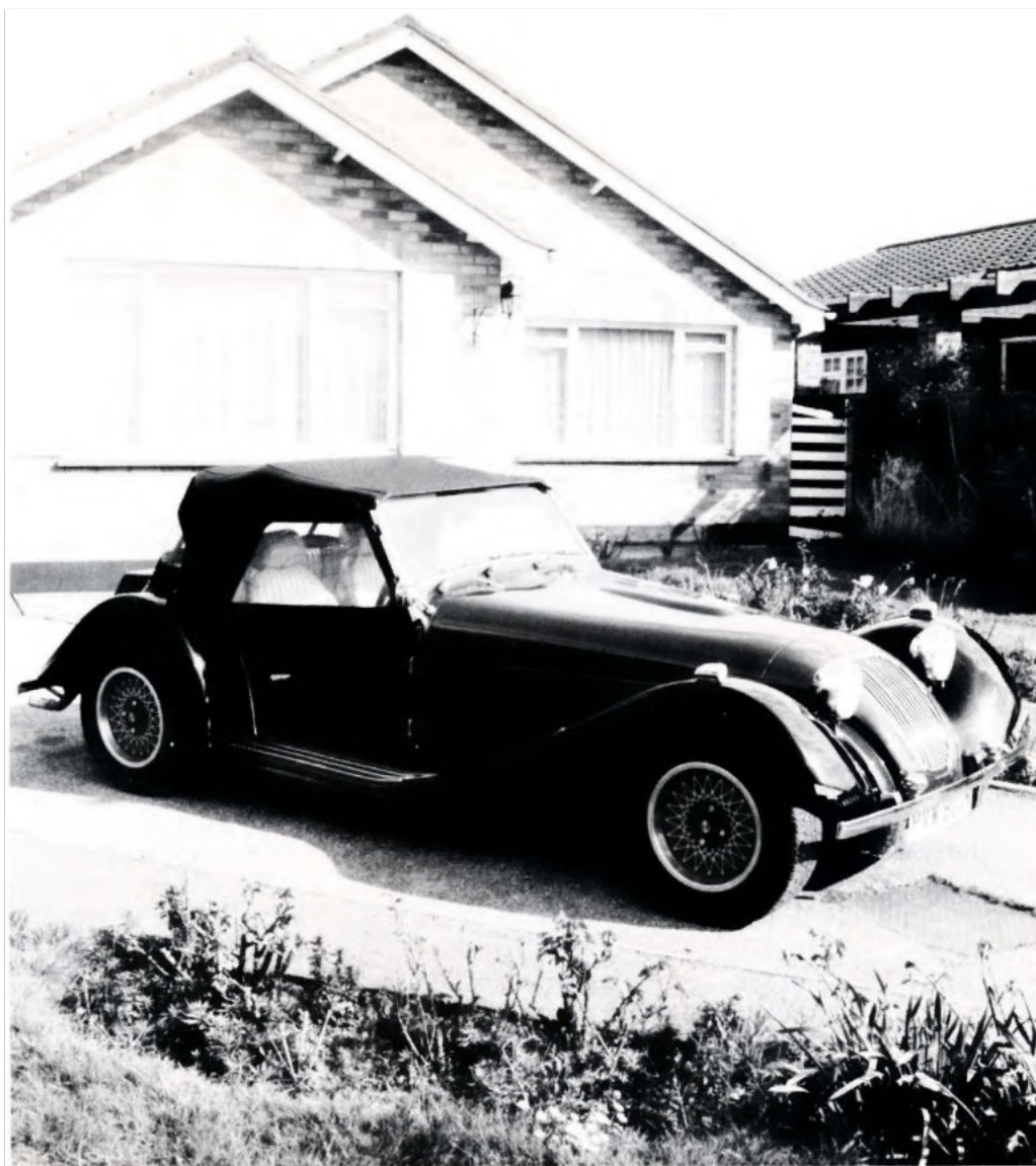
The hood fits extremely well and maintains the interior space with a high roof line and by fixing outside the elbow rests.
