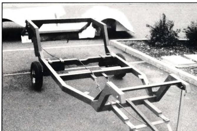
The simple, sturdy chassis supplied in primer. The wheels and bracket enable the kit to be towed home.
